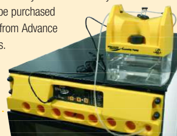
Humidity Pump Module connected
